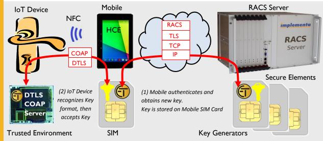
Providing ultimate end-to-end communication security between IoT devices, Mobile and Cloud applications. Communications are encrypted using TLS/DTLS. Certificates are stored in Secure Elements.
