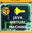
A Secure Element (SE) is a Secure Microcontroller, equipped with interfaces such as NFC, ISO7816, SPI or I2C. 9 billion of SE has been shipped in 2015, for SIM modules, bank cards, ePassport, PKI tokens.
