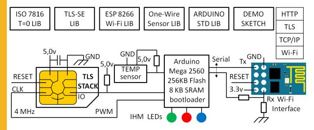
This use case demonstrates a low cost & low power, high security, Wi-Fi connected thermometer. All object communications go through the Secure Element and its imbedded TLS/DTLS stack.
