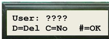
Type user on the Terminal emulator, to switch to user mode. The ECT will ask you to enter the user password, which is set for demonstration purposes at 0000 (4 zeros), then press #
