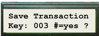
This means that: the transaction will use the key at Index 3, a nonce equal to 1, a Gas Price 30 GWEI, the GasLimit 30000, the Address 1BE31A94361A391BBAFB2A4CCD704F57DC04D4BB, the amount of the transaction 0.0 ETH, and the data included in the transaction the sentence "Hello Robert".
