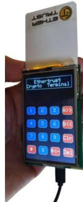
The Crypto Terminal is equipped with an *USB Serial* protocol, and a *Bluetooth Low Energy* (BLE) module with the RFCOMM profile. It includes a smartcard reader, and delivers the following services:
