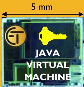
A Secure Element (SE) is a Secure Microcontroller, equipped with interfaces such as NFC, ISO7816, SPI or I2C. 9 billion of SE has been shipped in 2015, for SIM modules, bank cards, ePassport, PKI tokens.
